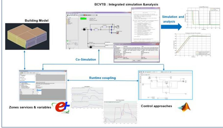
Figure 2: The integrated simulation and analysis of the state feedback technique
